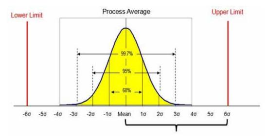
To calculate  $C_p$  and  $C_{pk}$  use the specifications and process widths. The specification width is the difference between the upper specification limit - Ls and the lower specification limit - Li, or the upper tolerance limit and the lower tolerance limit. If it is decreased, Ls - Li, the width of the specifications is obtained.
