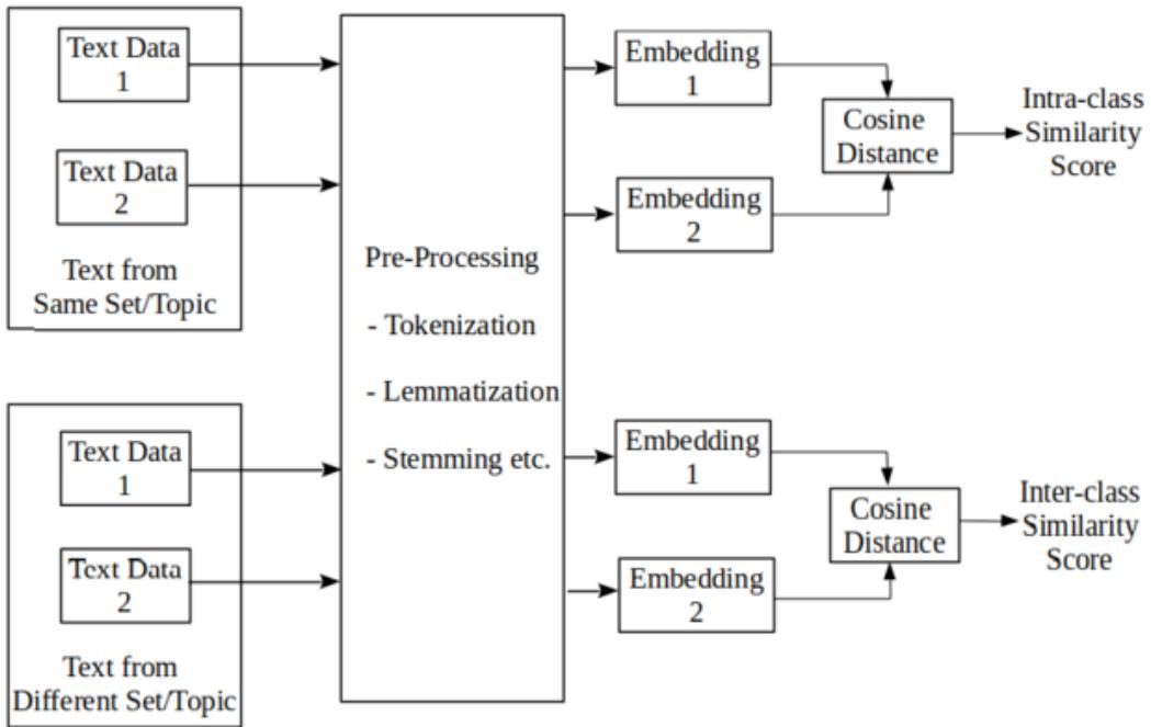
similarity metric to calculate the similarity between two set of texts. Cosine similarity computes the angle between the vectors representing the embeddings of two sets of text data.
